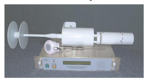
The Omnitech Electronics SM73 MDDS (Meteorological Data Distribution System) is a meteorological measurement system for shipboard installations. The MDDS was designed for the Canadian Navy's <u>Halifax Class</u> ships but can be customized by Omnitech for almost any application.
