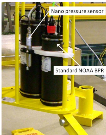
Figure 2. OSU/PMEL BPR/Tilt instrument showing relative placement of nano-resolution and standard BPR sensors.
