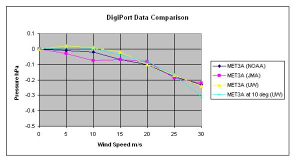
The second graph shows how much better the DigiPort (MET3A port) performs as compared to closely spaced dual disks, open pipes, or single plates at small pitch angle.
